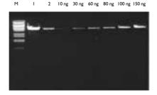
Quantities of extracted 4.5 kb DNA fragment corresponding to 1/5 of the DNA obtained by purification from 0.5 ug starting DNA with a recovery of 90 %. Sample were run on 1 % TAE agarose gel. M; Lambda-BstP1 marker Lane1; Total amount before extraction (0.5 ug) Lane2; 1/5 amount after extraction [90 ng compared to known amount ( $10 \sim 150$  ng) DNA] \* Total obtained amount of DNA =  $90 \times 5 = 450$  ng approximately (90 %)
