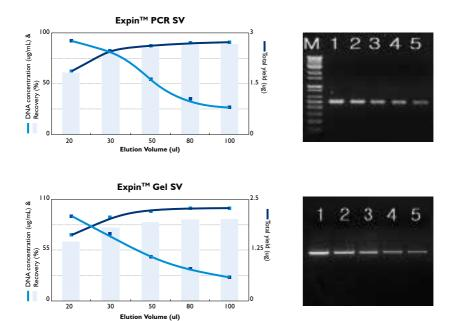
Correlation between the elution volume and the recover rates. Upper panel; GeneAll® PCR SV Kit. Lower panel; GeneAll® Gel SV Kit. 3 ug of 494 bp PCR products were purified and eluted with the indicated volumes of buffer EB. Elution volume lower than 30 ul causes significant loss of DNA. 1/10 volume of eluate purified with Gel SV Kit was resolved on 1 % agarose gel; lower right. (1/20 for PCR SV Kit, upper right)
